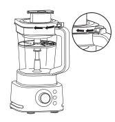
4 To install the feed chute lid on the jug, place the lid tab to the right of the handle. Press the lid down until it is secure. Rotate the tab clockwise until it clicks into place on the jug handle. Once the lid is locked in place, press the Power button to turn unit on.
