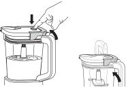
8 Remove the lid and Dough Blade Assembly before removing contents. To remove the lid, press the **RELEASE** button and lift the handle. To remove the blade assembly, carefully grasp it by the top of the shaft and pull straight up. The jug can then be emotied.
