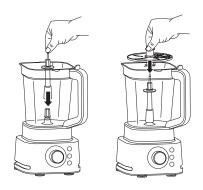
**3** Place the disc spindle onto the drive gear inside the jug. Then, use the plastic grip to grasp the disc and place it over the spindle.
