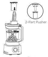
6 Add the prepped ingredients you want to slice or grate through the feed chute on the lid. Use the 2-part food pusher to help guide the food through the feed chute. The middle piece of the food pusher is removable to use for narrow ingredients.
