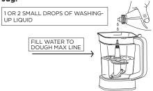
With the dough or stacked blade assembly installed, fill with warm water up to DOUGH MAX line and add 1 or 2 small drops washing-up liquid. Secure flat lid and ensure the pour spout is securely closed.
