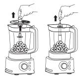
**9** Using the plastic grip, carefully lift the disc out of the jug. Then, grasp the spindle by the top of the shaft and lift it out of the jug.
