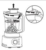
**8** To remove the lid from the jug, press the release button above the jug handle, and rotate the lid tab anti-clockwise out of the lock position, then lift the entire lid up.
