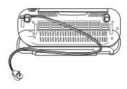
**Option 2:** Socket on the left or behind the toaster. Place the cord in both hooks on the back of the toaster. Twist the cord so the wide side is horizontal in order to securely fasten the cord in the hooks.
