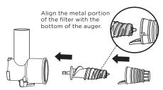
2 Insert the auger into the feed chute chamber, then attach the desired filter onto the auger, with the metal portion of the filter on the bottom of the auger.
