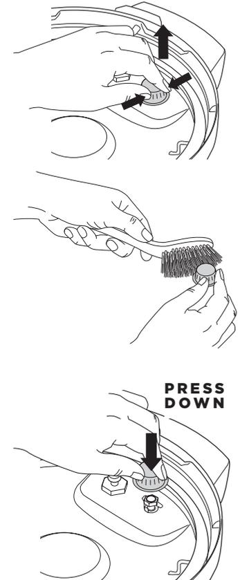
**NOTE:** Prior to each use, make sure the Silicone ring is well seated in the Silicone ring rack and the anti-clog cap is mounted properly on the pressure release valve.
