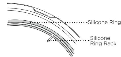
To remove the silicone ring, pull it outward, section by section, from the silicone ring rack. The ring can be installed with either side facing up. To reinstall, press it down into the rack section by section.
