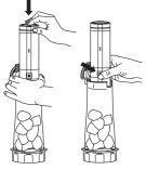
3 To vacuum-seal the cup, hold the pump in place over the seal. Press the power button on top of the pump once to begin vacuum-sealing. The light on the pump will illuminate in white while vacuum-sealing is in progress.
