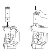
1 Set the pitcher on a level surface and place the FreshVac™ pump on top of the green vacuum release seal on the lid.
