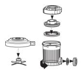
20 Rinse the outer bowl lid to remove any sticky residue or pieces wedged in the Swirl Creamerizer Paddle. Then detach the paddle by pressing the latch on the top of the outer bowl lid. For easy cleanup, release paddle directly into the sink.
