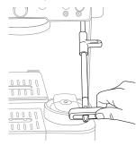
4 Use the needle to remove any material from inside the steam wand and steam wand tip.
