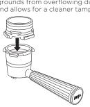
2 With the funnel on top of the portafilter, insert into the grinding cradle. Make sure it is level and fits securely. Once portafilter is installed in grinding cradle, it will be weighed. To ensure accurate weight, let go of portafilter.
