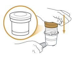
On a solid level surface with funnel still attached, press tamper all the
