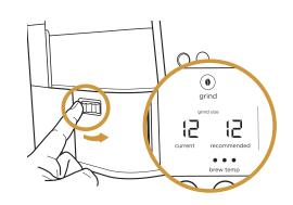
If they don't match, adjust current grind size by spinning the grind dial on left side of machine until it matches the recommended setting.
