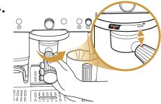
Fasten portafilter to align with lock arrow.
