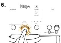
Press START BREW. The machine will beep to signal the brew has started. The progress bar will illuminate, indicating the status of the brew. This will take about 30 seconds.
