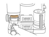
Insert portafilter in the grinding cradle. Make sure it is level and fits securely.
