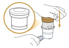
On a solid level surface with funnel still attached, press tamper all the way down until it meets funnel.
